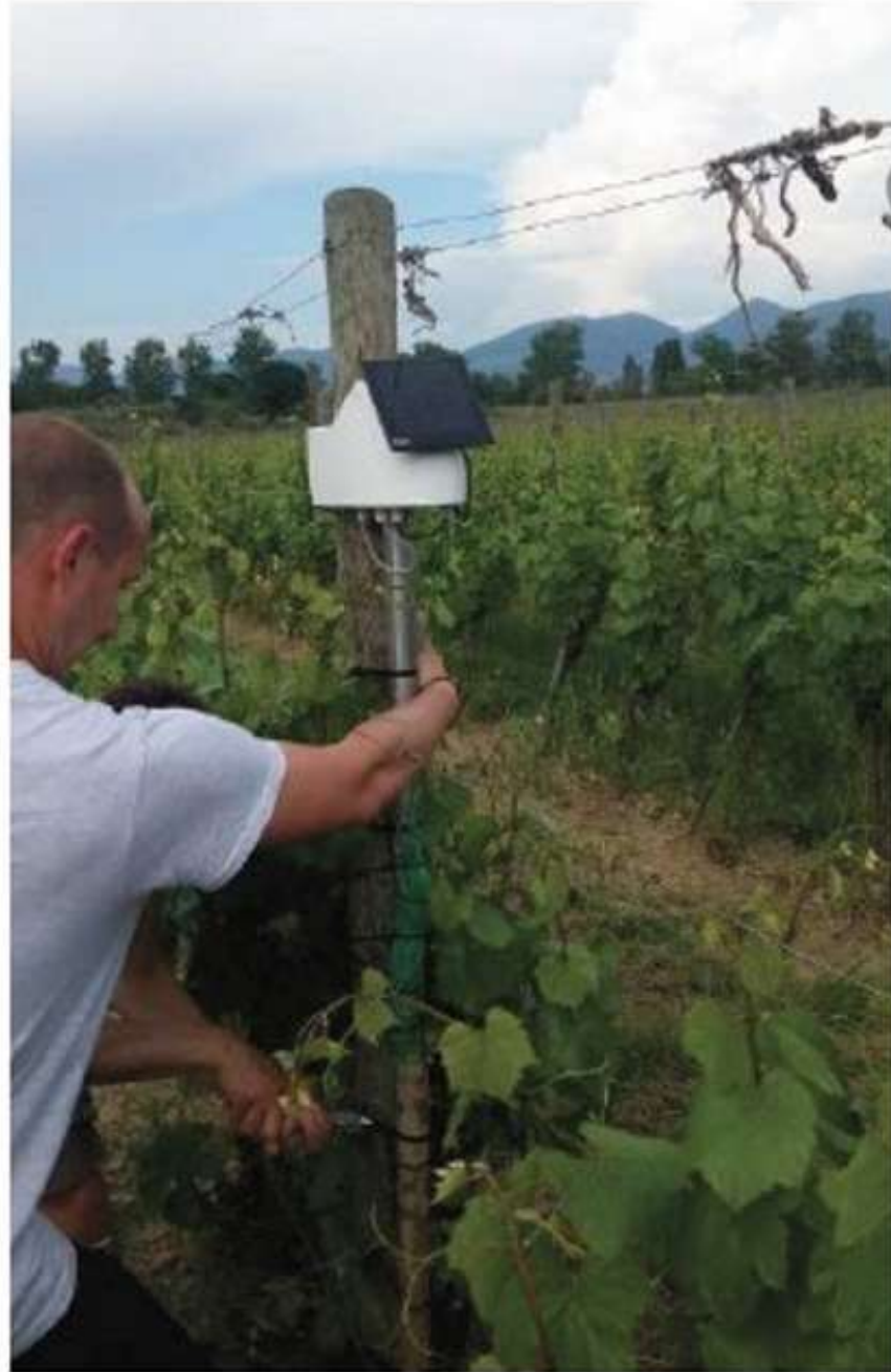
One of the dataloggers installed in a Chardonnay vineyard at Arnaldo Caprai in Umbria, Italy.
